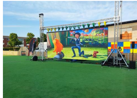
Screen Size: 21m 2 Pixel Pitch:3.91mm
