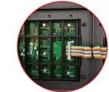
Signal cord with lock to avoid loose
