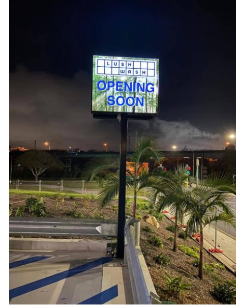
Screen Size: 1.1m 2 Pixel Pitch:3mm
