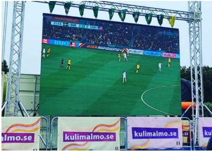
Screen Size: 15m 2 Pixel Pitch:3.91mm
