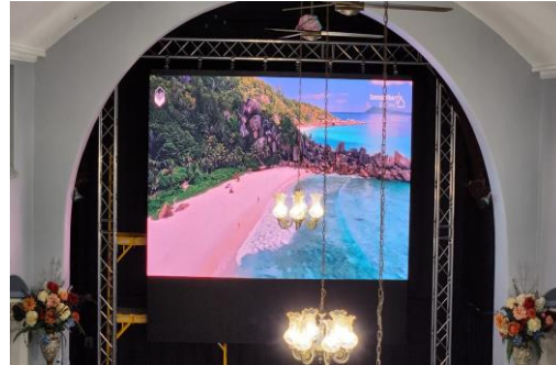
Screen Size: 10m 2 Pixel Pitch:3.9mm
