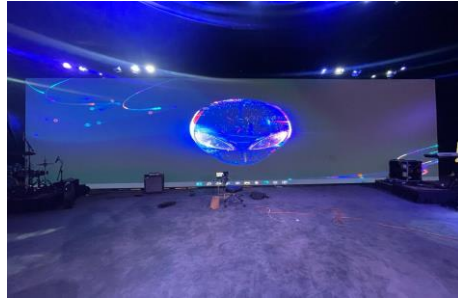
Screen Size: 87.5m 2 Pixel Pitch:2.9mm
